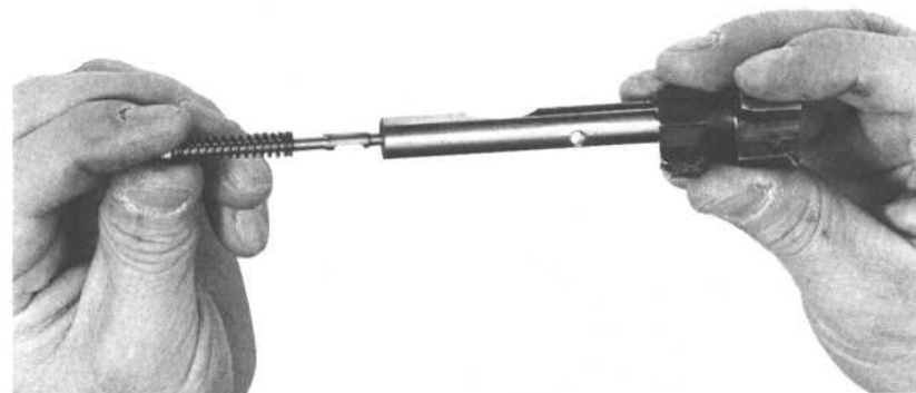
Install firing pin
