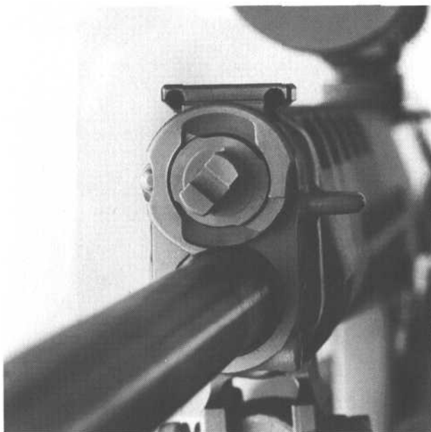
Gas valve on setting II
