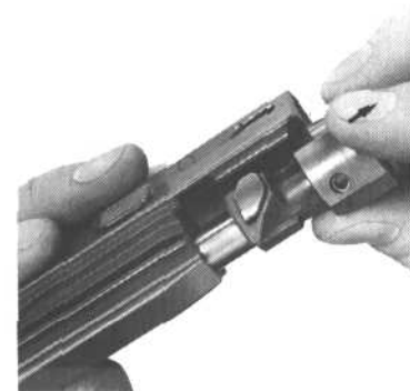
Remove bolt head
