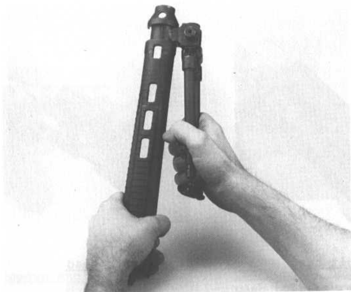
Remove bipod carrier
